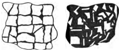
FIG. 12.—Sketches showing structure of breccia ore. (After Watson.) White areas, chert or sandstone; black areas, manganese ore. About one-fifth natural size.
